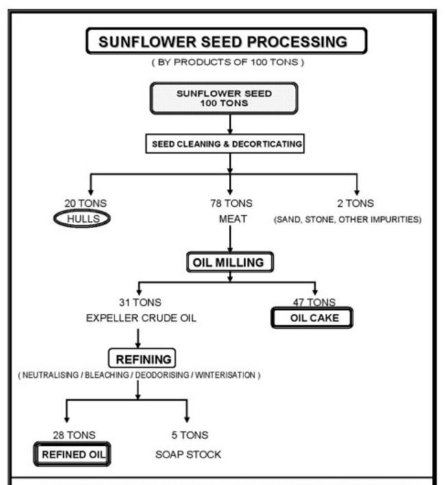
NOTE: THE FIGURES GIVEN HERE ARE APPROXIMATE AND MEANT ONLY TO HELP DECIDING THE BALANCED MATERIALS FOR PROCESSING UNITS TO BE INSTALLED SUCH AS OIL MILL, REFINING UNIT AS THE OIL CONTENT, PROTEIN, ETC. OF OIL BEARING MATERIALS VERY FROM SEASON, PLACE TO PLACE AND VARIOUS OTHER FACTORS.
