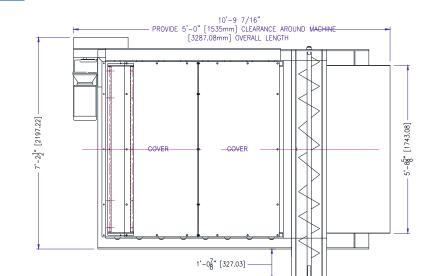
THE COTTOR / CANTRELL BEATER / SHAKER IS DESIGENED TO PRODUCE HULLS WITH A MINIMUM OIL CONTENT BY EFFICIENTLY BEATING THE HULLS TO REMOVE THE FINE, FLOURY AND SMALL PARTICLES OF MEATSAND OILY LINT.
