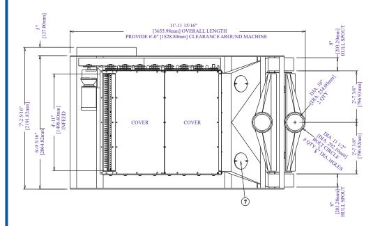
THE COTTOR / CANTRELL BEATER / SHAKER IS PRIMARY TO PRODUCE HULLS WITH A MINIMUM OIL CONTENT BY EFFICIENTLY BEATING THE HULLS TO REMOVE THE HIGH PROTEIN FINISHED MEATS.
