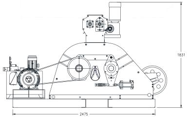
THE LARGE CAPACITY TWIN ROLL HULLER & BASKET BEATER / SHAKER IS PRIMARY TO PRODUCE HULLS WITH A MINIMUM OIL CONTENT BY EFFICIENTLY BEATING THE HULLS TO REMOVE THE HIGH PROTEIN FINISHED MEATS.
