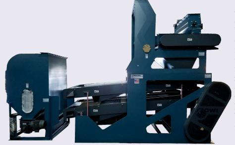
Oilseed processors demand quality and expect dependable equipment. Cantrell Worldwide demands dependability in each piece of equipment manufactured for the oilseed processing industry. The Cantrell Model 399 Cottonseed Cleaner is a complete unit designed to effectively remove foreign material from white cottonseed. Cottonseed cleaned through these machines produces cleaner lint, higher cellulose content and allows for better Delinting and Dehulling (Decorticating).
