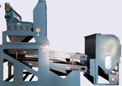
bolls, stems, sticks etc., across to screen, while shifting out small bran dirt, fines across bottom pan, and discharging screened seed into a large rock trap cleaner. The rock trap cleaner not only separates rocks, metal, bolts and heavy contamination, but it also lifts out any remaining, loose lints, dust, bran and light hulls, leaving a clean finished seed stream, putting quality into the entire process.
