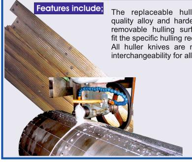
The replaceable huller knives are manufactured from the highest quality alloy and hardened to  $52R^c$  for extra long process life. Having removable hulling surfaces allows Cottor to tailor the knife profiles to fit the specific hulling requirements of the wide variety of oil seeds processed. All huller knives are manufactured from a single fixture giving absolute interchangeability for all replacements.
