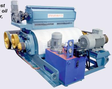
The heart of the hulling process is the twin, rugged 18" dia rolls equipped with removable huller knives. These twin rolls are driven at a ratio to enhance the cutting process thus minimizing the amount of uncut and recycle seed. This ratio combined with a spiral lead on the cutting edges allows the highest percentage of open "hulled" seed available to the separation room.
