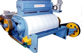
THE 36" TWIN ROLL HULLER & BASKET BEATER / SHAKER IS PRIMARY TO PRODUCE HULLS WITH A MINIMUM OIL CONTENT BY EFFICIENTLY BEATING THE HULLS TO REMOVE THE HIGH PROTEIN FINISHED MEATS.
